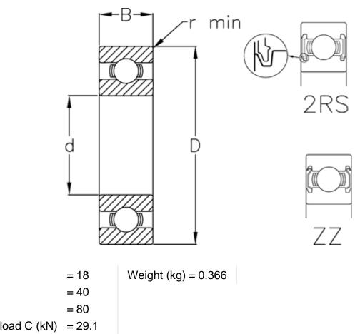
Dynamic load C (kN) = 29.1 Max rpm greased = 8700 Max rpm oil lubricated = 10000 r min = 1.1 Static load C0 (kN) = 17.8
